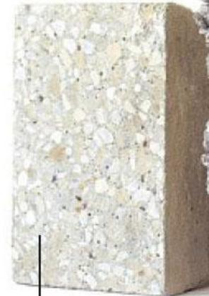
Gravel or crushed stone mixed with cement, water and sand.
