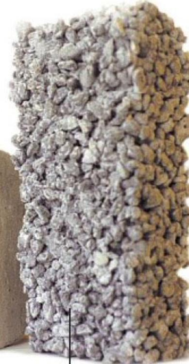
Uses stone that is smaller than conventional concrete and cement with little or no sand in the mixture. This creates porous spaces that allow water to pass through.
