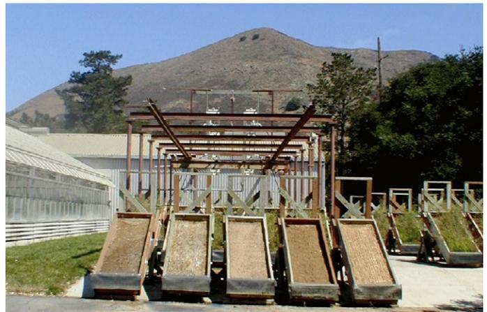
**Figure 1. Test boxes at 2H:1V south-facing slope.**
