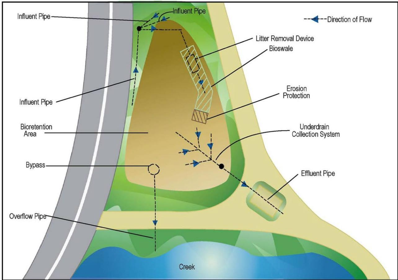
**Figure 2 Plan View of the Original Bioretention Design**
