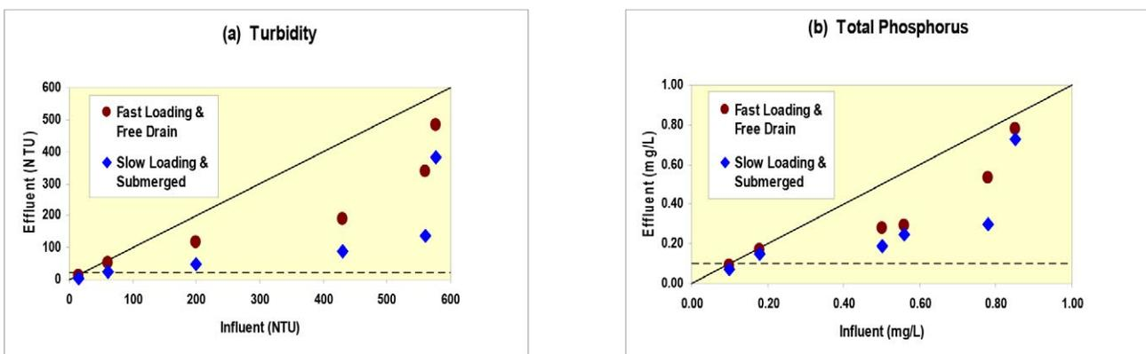
**Figure 5 Effect of filter loading conditions – comparison of fast loading/free-drain and slow loading/submerged for (a) turbidity and (b) total phosphorus. (Dotted lines represent surface discharge limits and solid diagonal lines represent no treatment).**
