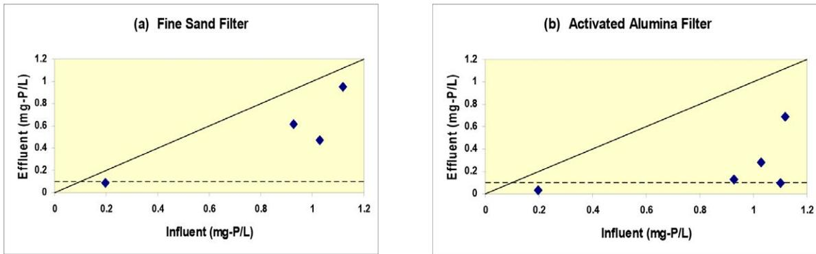
**Figure 4 Total phosphorus removal results for (a) fine sand and (b) activated alumina filtration for Year 1 (no sedimentation, fast loading, free-drain). (Dotted lines represent surface discharge limits and solid diagonal lines represent no treatment).**
