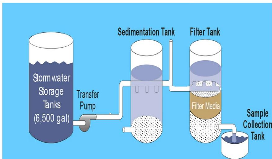
**Figure 2 Schematic of a Sedimentation/Filtration System**
