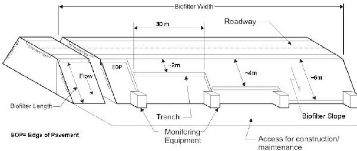
**Figure 1. Schematic of Collection System**
