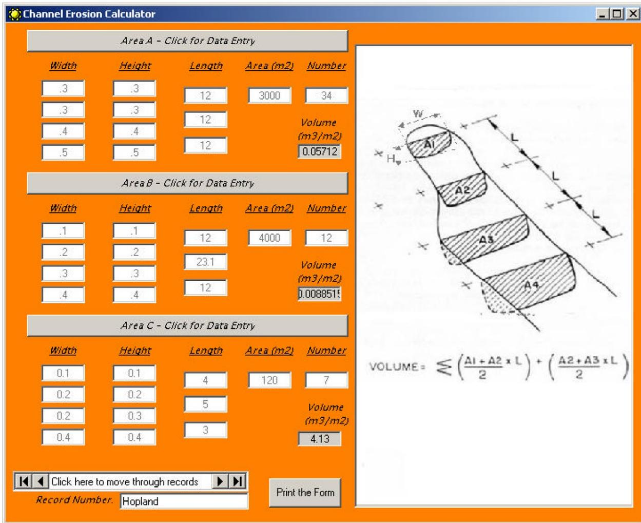
**Figure 5. Channel calculations are performed for up to three areas of the site (channel diagram adapted from Hudson, 1995).**
