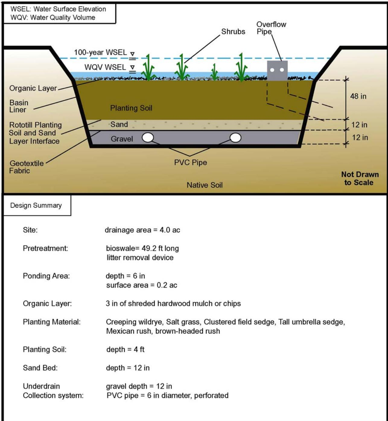
Figure 1 Cross Section and Summary of Original Bioretention Design
