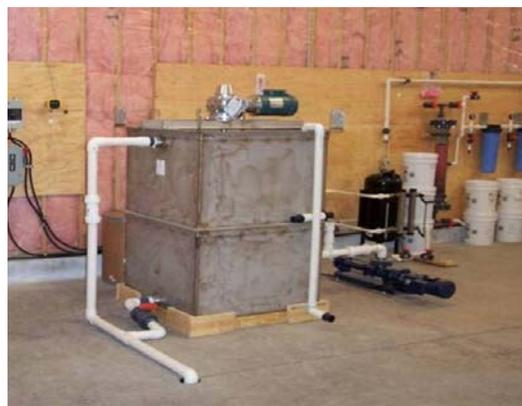
Figure 2. Batch reactor for the mechanized treatment systems. The dark canister to the right is the pressure sand filter.
