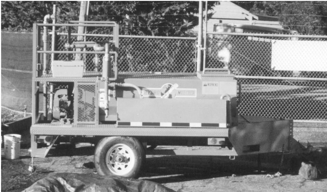
Figure 1. 600-gallon hydromulcher used to apply mulch materials
