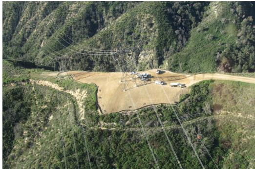
**Figure 14: This site does not qualify for final stabilization. The surrounding vegetation indicates very dense pre-project vegetation coverage. The postconstruction sediment delivery is substantially higher than the pre-project condition due primarily to the lack of postconstruction vegetation relative to preconstruction.**
