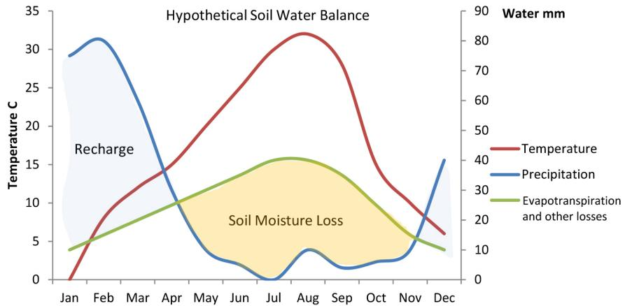
**Figure 3: Soil Water Balance**
