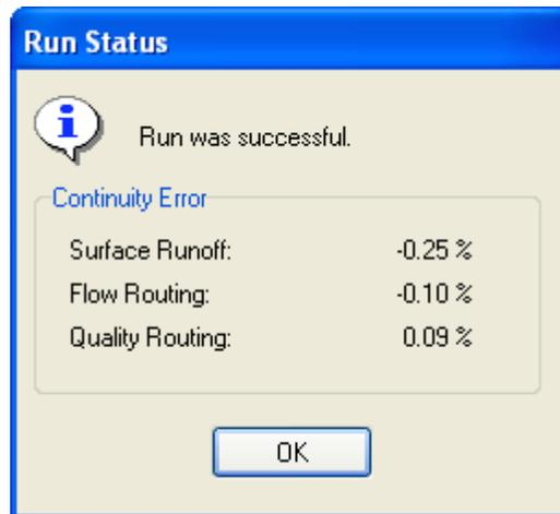
In addition to the system continuity error, the Status Report produced by a run (see Section 9.1) will list those nodes of the drainage network that have the largest flow continuity errors. If the error for a node is excessive, then one should first consider if the node in question is of importance to the purpose of the simulation. If it is, then further study is warranted to determine how the error might be reduced.
