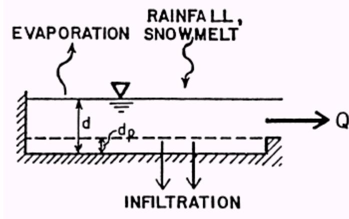
Figure 3-6. Conceptual view of surface runoff.
