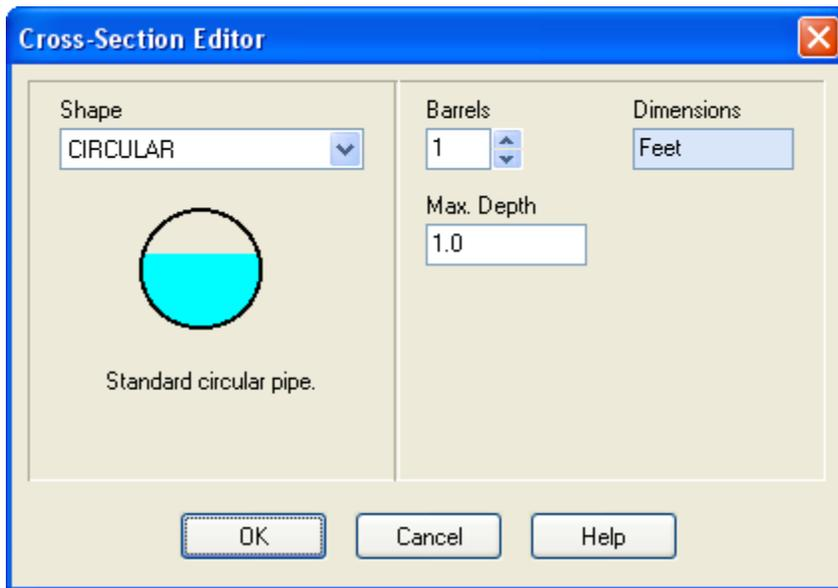
The Cross-Section Editor dialog is used to specify the shape and dimensions of a conduit's cross-section. When a shape is selected from the dropdown combo box an appropriate set of edit fields appears for describing the dimensions of that shape. Length dimensions are in units of feet for US units and meters for SI units. Slope values represent ratios of horizontal to vertical distance. The Barrels field specifies how many identical parallel conduits exist between its end nodes.
