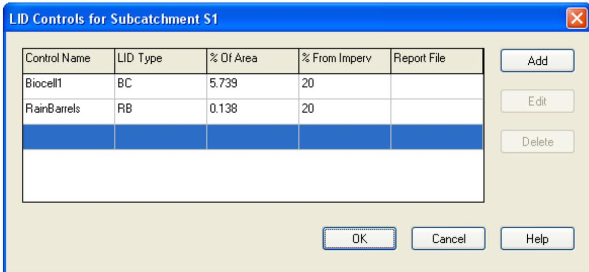
The LID Group Editor is invoked when the LID Controls property of a Subcatchment is selected for editing. It is used to identify a group of previously defined LID controls that will be placed within the subcatchment, the sizing of each control, and what percent of runoff from the non-LID portion of the subcatchment each should treat.
