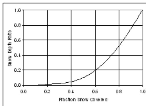
**Figure 3-2. Areal Depletion curve for a natural area.**
