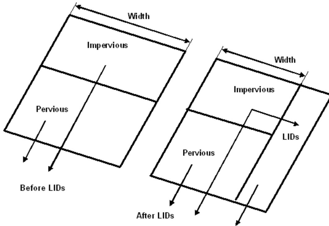
Figure 3-5. Adjustment of subcatchment parameters after LID placement.
