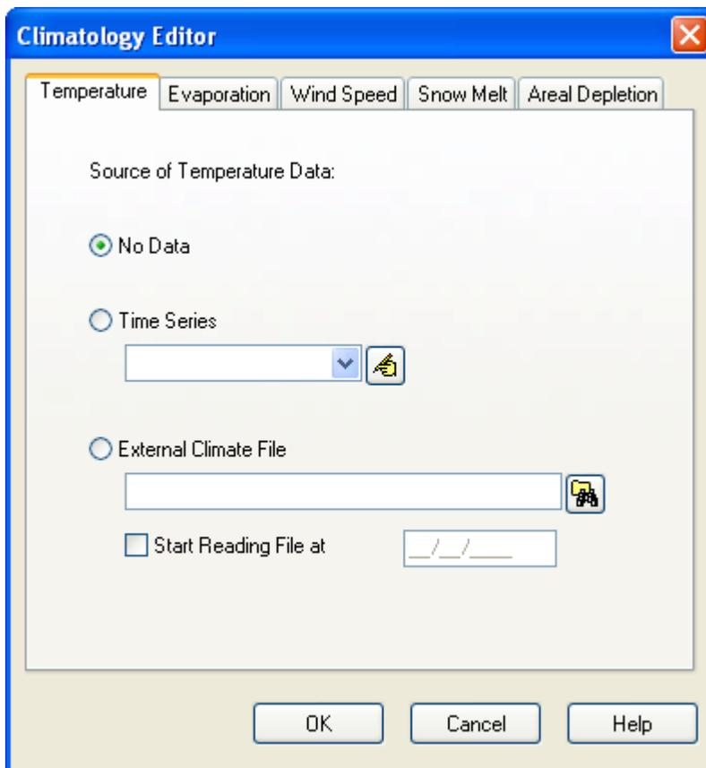
The Temperature page of the Climatology Editor dialog is used to specify the source of temperature data used for snowmelt computations. It is also used to select a climate file as a possible source for evaporation rates. There are three choices available:
