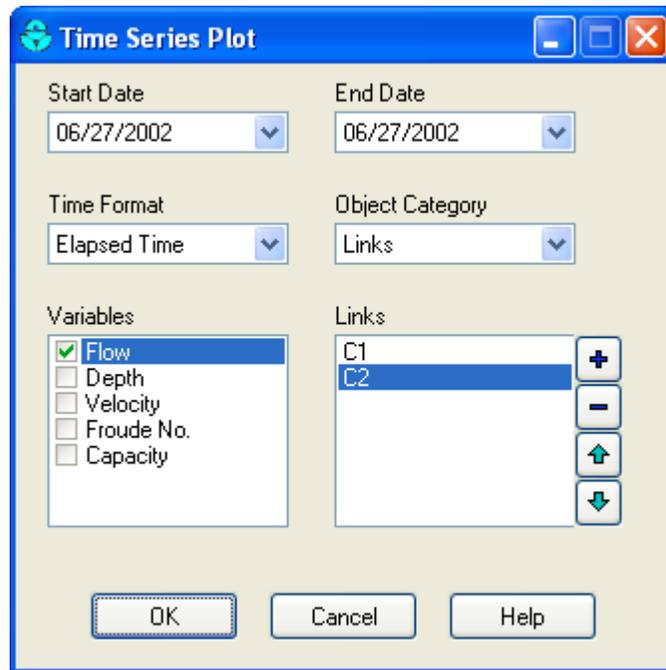
The Time Series Plot dialog describes the objects and variable to be graphed in a time series plot. Time series for certain system-wide variables, such as total rainfall, total runoff, total flooding, etc., can also be plotted. Use the dialog as follows:
