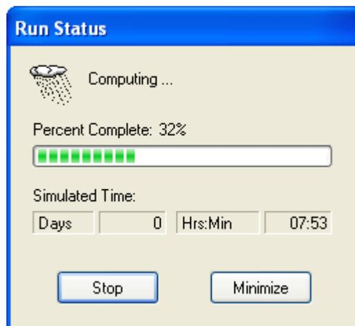
To stop a run before its normal termination, click the **Stop** button on the Run Status window or press the <Esc> key. Simulation results up until the time when the run was stopped will be available for viewing. To minimize the SWMM program while a simulation is running, click the **Minimize** button on the Run Status window.
