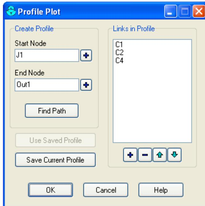
The Profile Plot dialog is used to specify a path of connected conveyance system links along which a water depth profile versus distance should be drawn. To define a path using the dialog:
