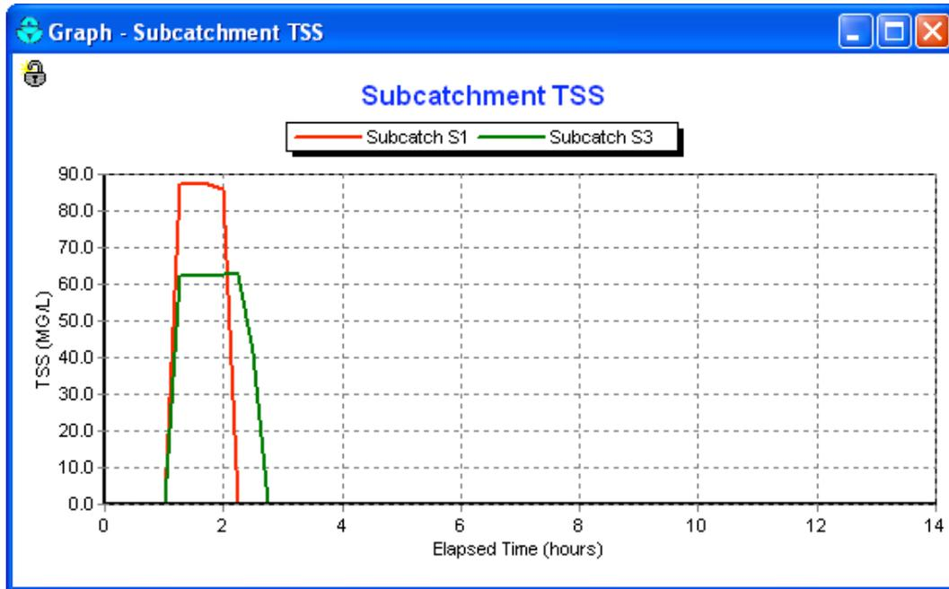
**Figure 2-21. TSS concentration of runoff from selected subcatchments.**
