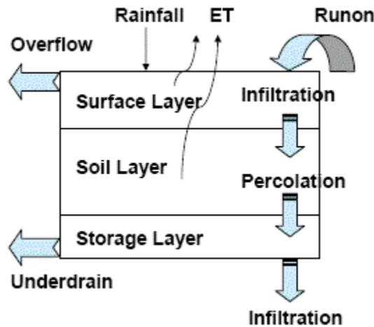
Figure 3-8. Conceptual diagram of a bio-retention cell LID.
