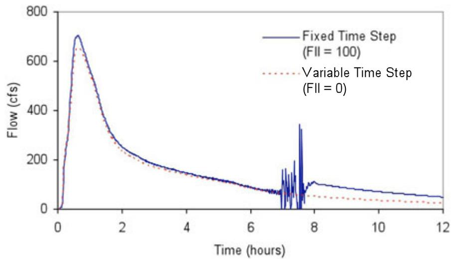
Flow time series plots for the links having the highest FII's should be inspected to insure that flow routing results are acceptably stable.
