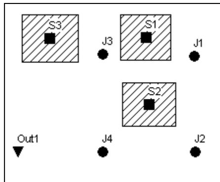
**Figure 2-4. Subcatchments and nodes for example study area.**
