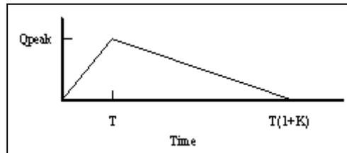
**Figure 3-3. An RDII unit hydrograph**
