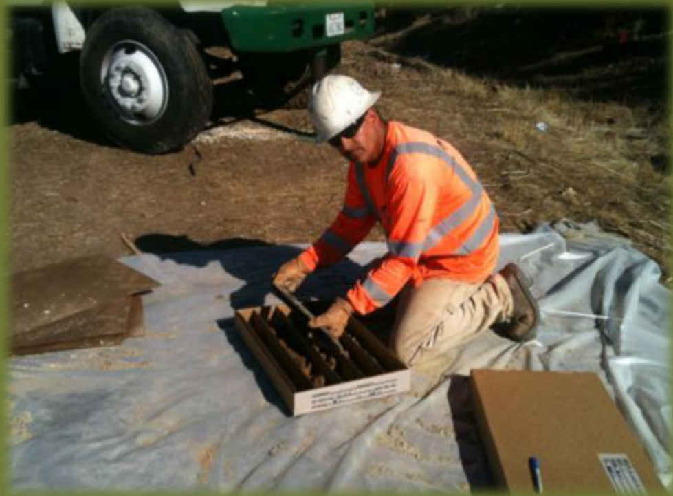
Logging boring soil samples at well sites
