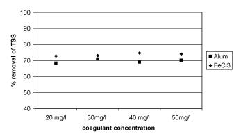
Figure 3—TSS removal efficiency with coagulant dose for ferric chloride and alum.
