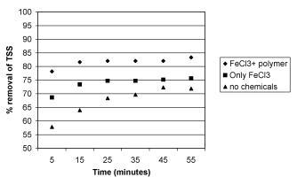
Figure 2—Selection of settling time.
