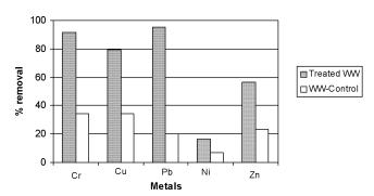
Figure 6—Comparison of chemically treated sample with control.
