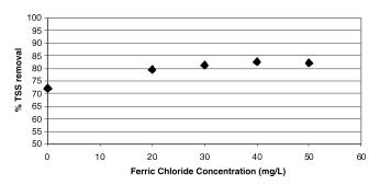
Figure 4—TSS removal efficiencies using ferric chloride with 0.5 mg/L polymer.
