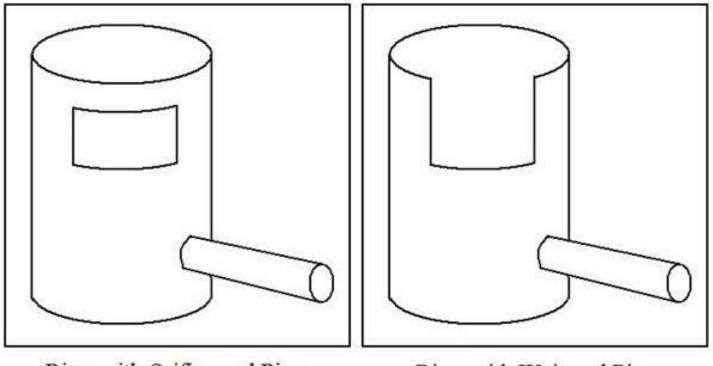
Riser with Orifice and Pipe Outlet Control Riser with Weir and Pipe Outlet Control
