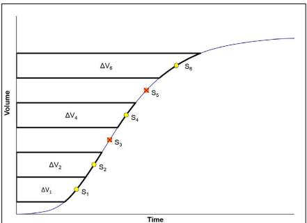
$$V_{rep} = \sum_{i=1}^{m} \Delta V_i = \Delta V_1 + \Delta V_2 + \Delta V_4 + \Delta V_6$$
