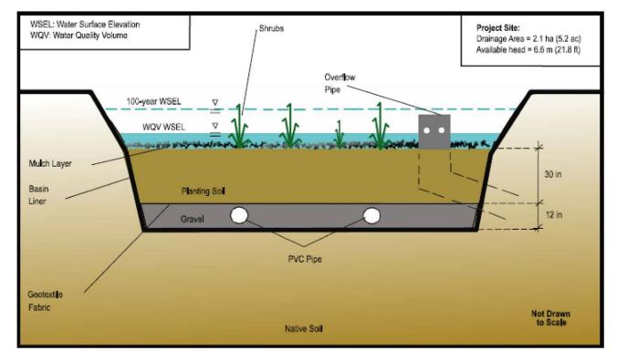
Figure 1. Cross-sectional view of bioretention area.
