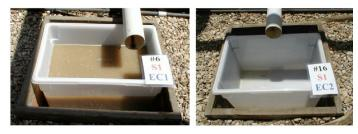
Figure 10. Runoff collection bins: S1 control (left) and S1 seed in 1680 kg/ha fiber with no compost (right).
