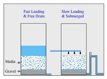
Figure 3 Schematic of fast loading/free drain and slow loading/submerged filter operating conditions
