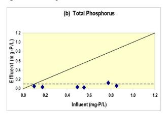
Figure 7 Expanded shale filtration results for (a) turbidity and (b) total phosphorus (slow loading, submerged, following 24-hour sedimentation). (Dotted lines represent surface discharge limits and solid diagonal lines represent no treatment).
