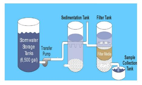
Figure 2 Schematic of a Sedimentation/Filtration System
