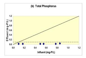
Figure 6 Activated alumina filtration results for (a) turbidity and (b) total phosphorus (slow loading, submerged, following 24-hour sedimentation). (Dotted lines represent surface discharge limits and solid diagonal lines represent no treatment).
