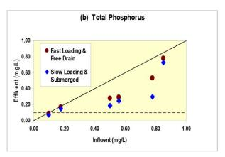
Figure 5 Effect of filter loading conditions – comparison of fast loading/free-drain and slow loading/submerged for (a) turbidity and (b) total phosphorus. (Dotted lines represent surface discharge limits and solid diagonal lines represent no treatment).
