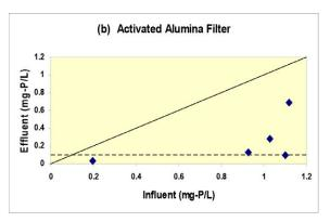
Figure 4 Total phosphorus removal results for (a) fine sand and (b) activated alumina filtration for Year 1 (no sedimentation, fast loading, free-drain). (Dotted lines represent surface discharge limits and solid diagonal lines represent no treatment).
