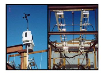
Figure 3. Weather station and rainfall simulators.
