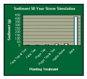
Figure 5. Sediment load 50-year storm simulation.
